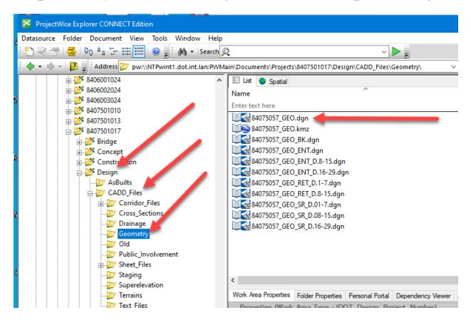
This is the container GEO file that will contain all the Alignments for this project. Attach it using the orientation of Coincident World. Turn on the live nesting and set its depth to 1.
