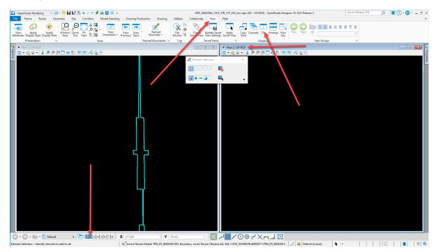
Open the View Attributes tool in view 2. Select the CIP RCB-3D model in the View Setup section of the View Attributes tool.
