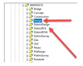
For this example, it is being done by the Design group. So the corridor file is under the CADD\_Files\ Corridor\_Files\folder. Select the COR Corridor file that is named COR\_CCRRRPPPZZZ.dgn.
