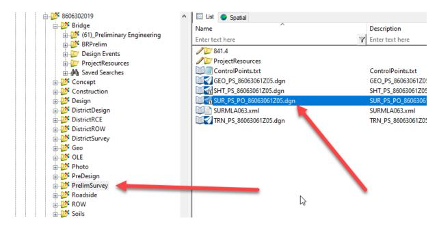
Next reference in the Design alignment that has an active profile. This file should be located in the Design or the District Design folder (depending what group is doing the road design portion of this project).
