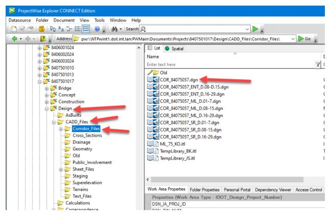
This is the container COR file that will contain all the Corridor for this project. Attach it using the orientation of Coincident World. Turn on the live nesting and set its depth to 1.
